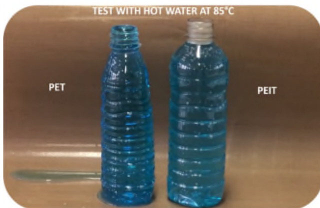
Figure 2: PEIT grades exhibit much less shrinkage than PET when subjected to temperatures comparable to those associated with hot fill.
