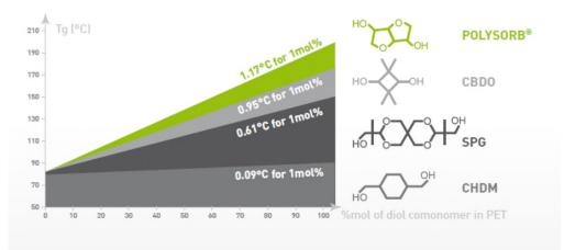
POLYSORB<sup>®</sup>, the high purity isosorbide from Roquette, is the most effective diol for increasing the Tg of specialty copolyesters and a bio-based molecule.
