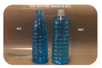
PEIT grades exhibit much less shrinkage than PET when subjected to temperatures comparable to those associated with hot fill.
