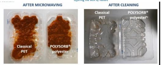
PEIT trays holding Bolognese sauce show no distortion or discoloration after 30 seconds in the microwave at 900W, unlike PET trays which are perform poorly in this application.
