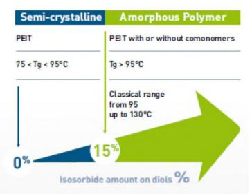
PEIT for aerosol packaging requires less than 15% isosorbide and is therefore semicrystalline. enabling recycle into existing PET streams.
