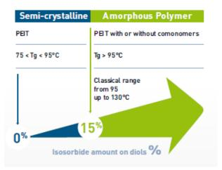
Incorporating isosorbide addresses an important constraint of PET, efficiently increasing T<sub>g</sub>.
